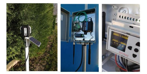
**Smart irrigation** systems tailor watering schedules and run times automatically to meet specific landscape and crop needs. These applications significantly improve outdoor water use efficiencies. Unlike traditional irrigation controllers that operate on a preset programmed schedule and timers, smart irrigation controllers may monitor weather, soil conditions, evaporation and plant water use to automatically adjust the watering schedule to actual conditions of the site.
