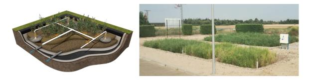
Constructed wetlands are filters composed of gravel and sand of different granulometry and planted on the top layer with local plants (usually Phragmites), They make use of filtration and biological treatment processes to provide treatment for urban wastewater.
