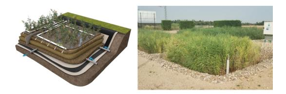
VFCWs can be used as a **second stage** of a 2-stage VFCW system or after a PUSH system for pretreatment. Gross solids are removed in the first stage, so the VFCW system can use sand as the top layer since there is a lower risk for clogging of the surface. Sand allows to increase wastewater retention time, allowing a larger contact time with the microbial community in the filter who will treat soluble organic matter and nutrients.
